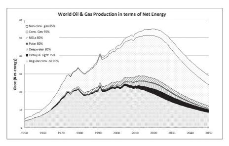
**Figure 2:** The same data as Figure 1, but now expressed in terms of 'net-energy barrels of oil equivalent' (i.e., barrels of useful energy delivered to society), once the energy used in the production of the oil and gas is subtracted off.
