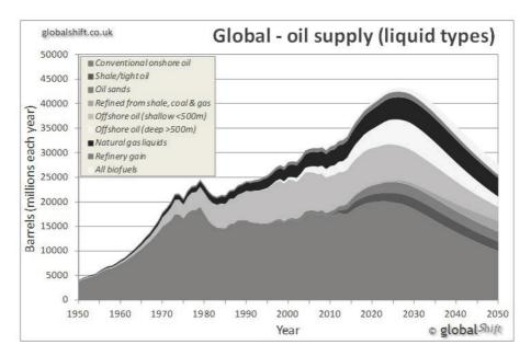
**Figure 6:** Historical data, and forecast, of all liquid types through to 2050. Shale/ tight oil, oil sands and refined liquids act to maintain onshore output to the end of the 2020s, whilst new production from progressively deeper waters sustains offshore output. government policy, especially since many economists and academics who engage in advising managers and governments have never worked in the oil exploration or production business.
