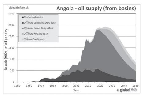
**Figure 2:** Historical data, and forecast, of oil supply in Angola, 1950 - 2050, by basin (including NGLs). The development of technologies to exploit deep water oil and more recently to image sub-salt has dramatically improved Angola's potential, such that all its offshore basins are now being explored and/or exploited.
