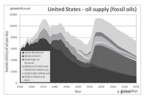
**Figure 1:** Historical data, and forecast, of all fossil oil production in the USA, 1950 – 2050 (includes shale/tight oil, oil sands and NGLs; excludes GTLs, CTLs & biofuels). For this oil, the USA will have 3 peaks: 1st driven by conventional onshore oil in 1970; 2nd driven by new Alaskan output in 1985; 3rd through a combination of shale oil, deep-water oil and NGLs around 2020
