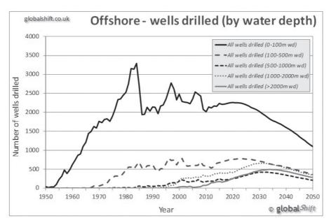
**Figure 3:** Historical data, and forecast, of global offshore drilling 1950 - 2050 by water depth. Drilling totals are dominated by shallow wells (drilled with jackups). Relative future growth is expected in ultra-deep waters (drilled with high-specification mobile rigs).
